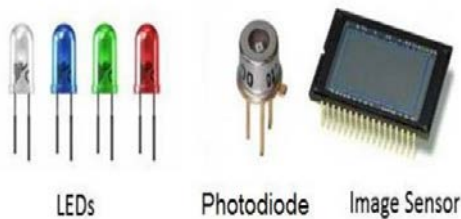
Fig 5. Components of Li-Fi system
